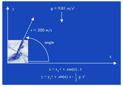
where  $x_0$  and  $y_0$  are the initial position (can be considered as 0 for both), and  $\alpha$  is the angle in radians ( $\Pi$  radians = 180°).
